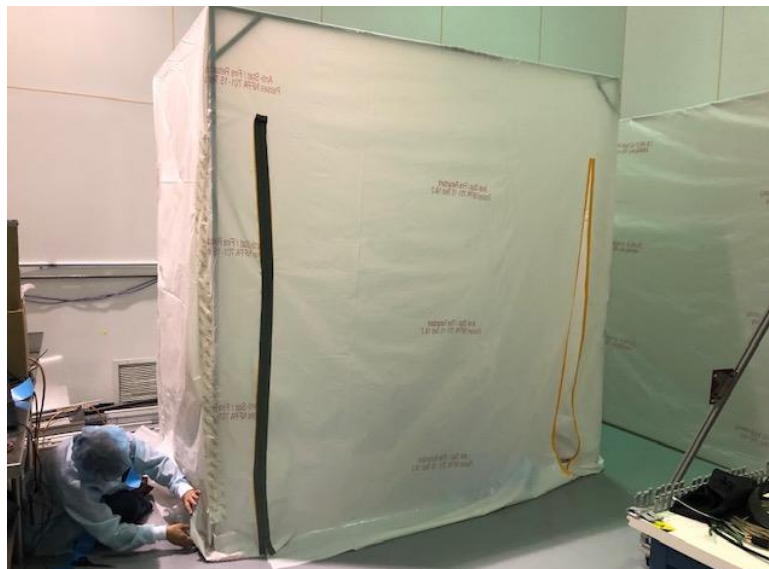
Mindy Leffel adjusting the flame-retardant plastic on the second Aerogel dry-tent
